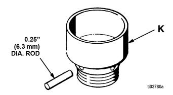
**NOTE:** Over tightening the Packing Nut/Wet-Cup (K) can cause premature wear and reduce system performance.
