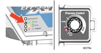
Rapidly cycle the Power Switch (C) from OFF to ON 12 times within 10 seconds.
