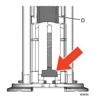
4. Slide the Driver (AA) onto the Pump Lower (AB). The notch in the ProConnect Coupler (H) should align with the button head on ProConnect Pump Rod (L).
