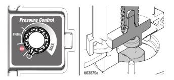
**NOTE:** If Driver (AA) failed to park this could be due to reaching maximum fluid pressure of the system. Hold a metal part of the spray gun/dispense valve to the side of a grounded metal pail and trigger the gun/dispense valve.
