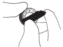
Fig. 19: Unthread Cap from PCD Body
