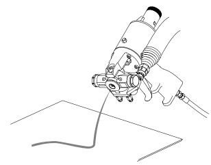
Fig. 2: Trigger Gun to Relieve Pressure
